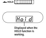
You can use the HOLD function with both the CD player and remote control. You can still operate your CD player using the remote control when HOLD on the remote control is set to off
